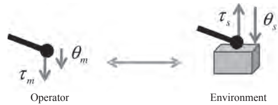
Figure 6: Basics of bilateral control
