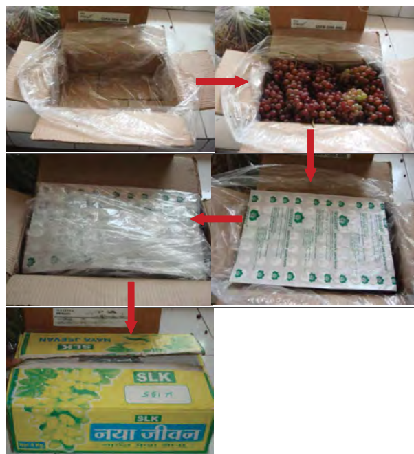
Figure 3: Packaging in corrugated fibre board boxes with polyethylene liner and a grape guard
