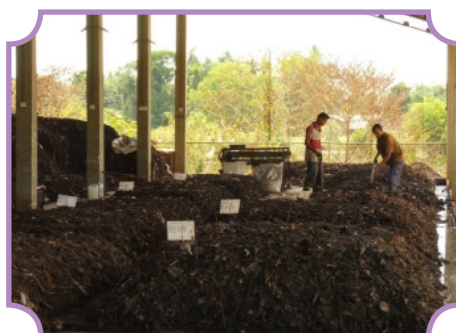
Figure 9 : Static pile & Windrow
